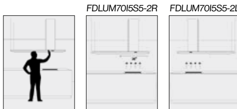
Right hand side example: chimney and button boards are on the right side when standing in front of the hood.
